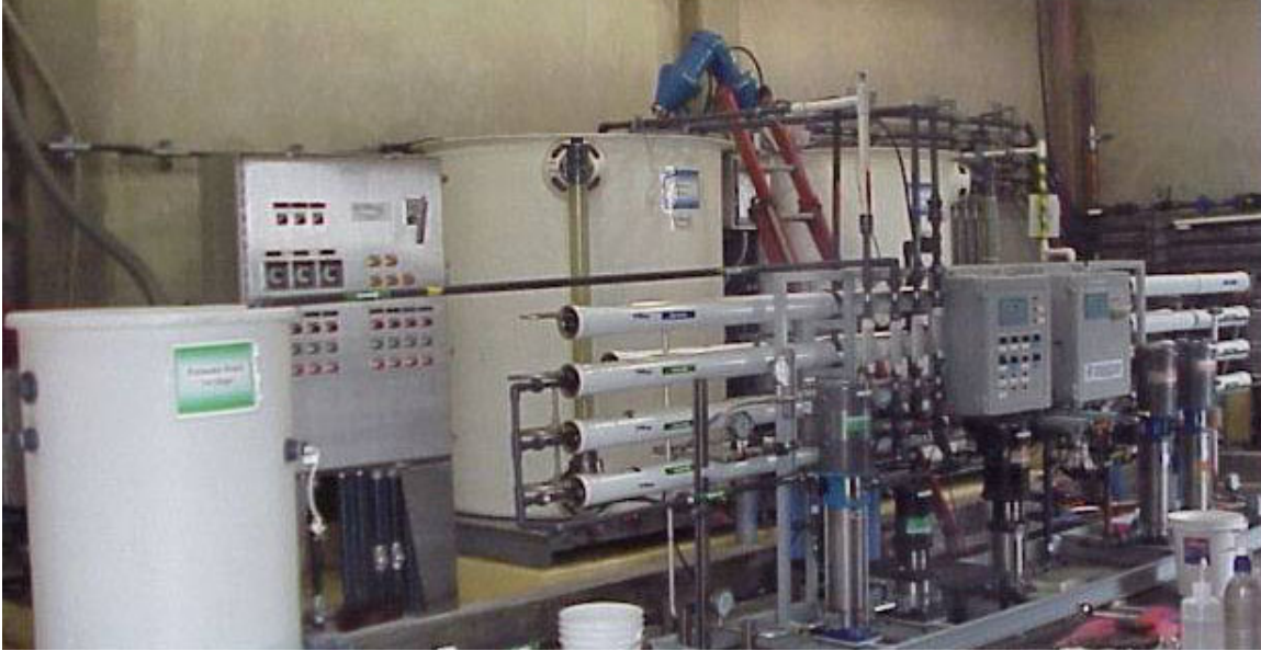
Figure 1. Photo of pilot plant used to test nanofiltration membranes for seawater desalination.
