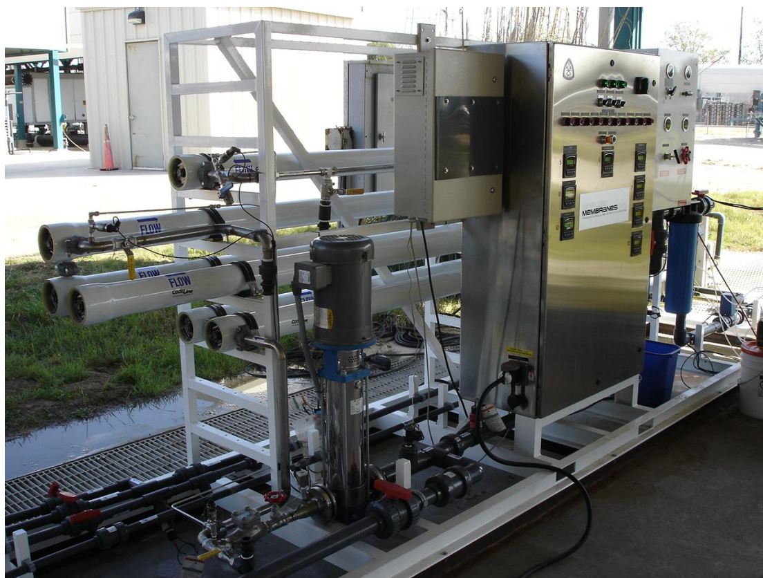
Figure 2. NF/RO Pilot-scale Skid employed during study
