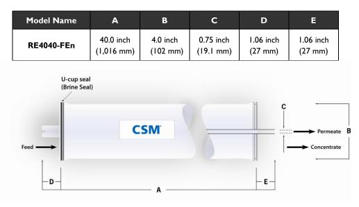
Each membrane element supplied with one brine seal, one interconnector (coupler) and four o-rings.
